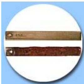
Corrosion Coupon Analysis
